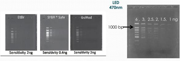
The best sensitivity (1 ng) when MaestroSafe is used combined with MaestroGen LED Transilluminator.
