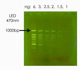
The best sensitivity (1 ng) when MaestroSafe™ is used combined with MaestroGen LED Transilluminator.
